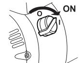
4. Turn the Engine Switch on.
